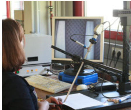
Testing of carbide inserts in needle holders
